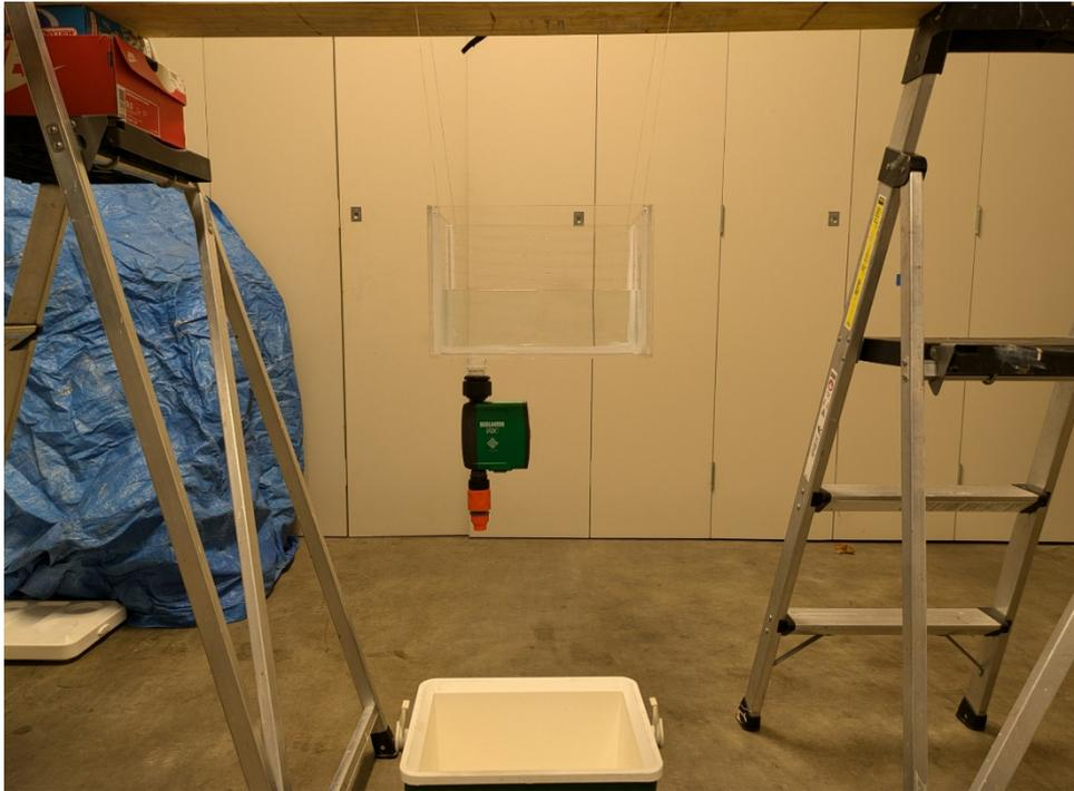
*Figure 5.18: The experimental set up, including the tank being suspended from a wooden beam and a container placed below the tank to catch the water released.*
