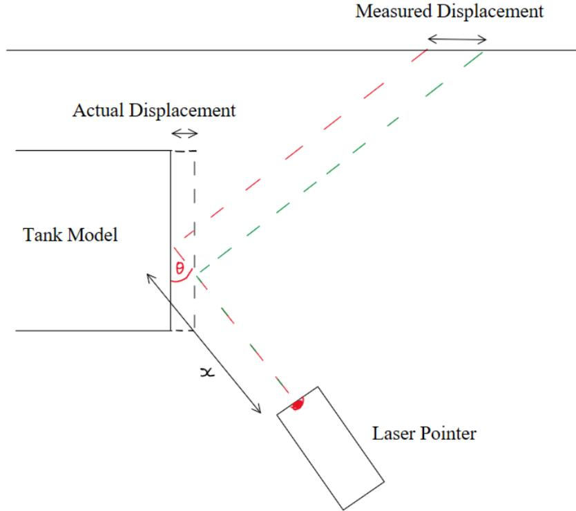
Figure 5.20: Top-view diagram of the experimental setup used to measure the displacement of the tank.
