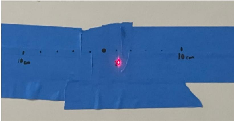
Figure 5.21: The point of the laser measurer reflected onto the back wall during the 12 mm outlet diameter testing.
