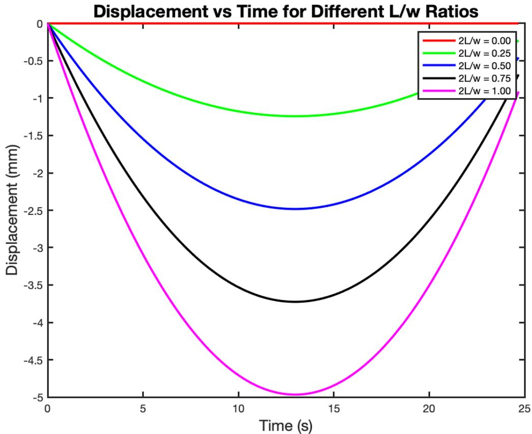
Figure 5.6: Graph of displacement against time for various  $L/W$  ratios.
