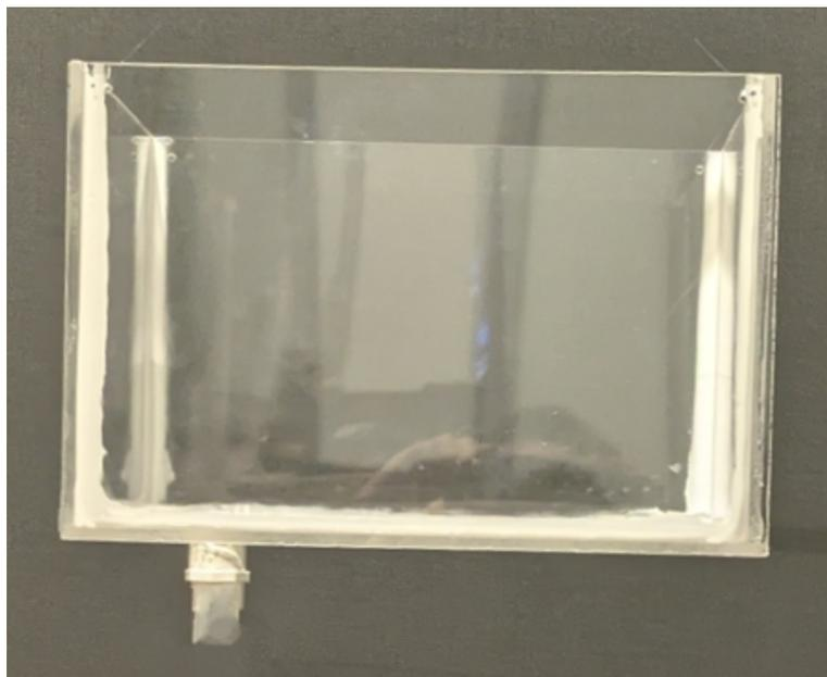
*Figure 5.17: The completed experimental tank with silicone applied, now ready to be used in testing.*
