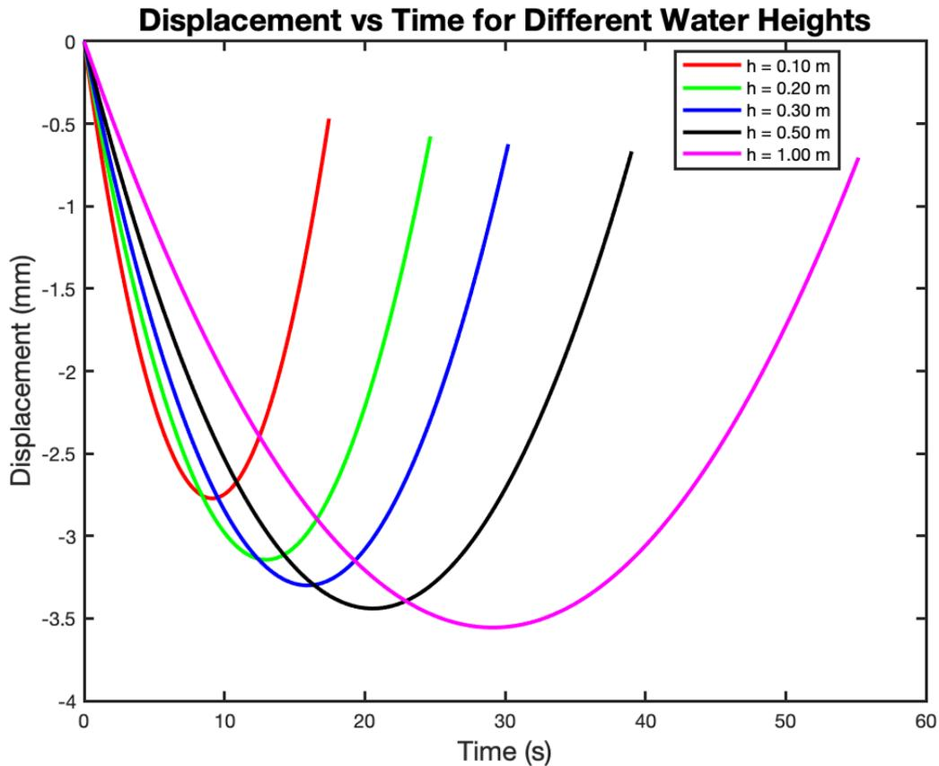
Figure 5.3: Graph of displacement against time for various water level heights.
