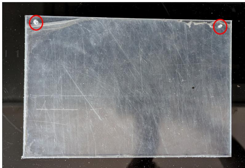
*Figure 5.13: An acrylic panel exhibiting two small holes on the top corners (circled in red) used to loop fishing line through to hold the tank.*
