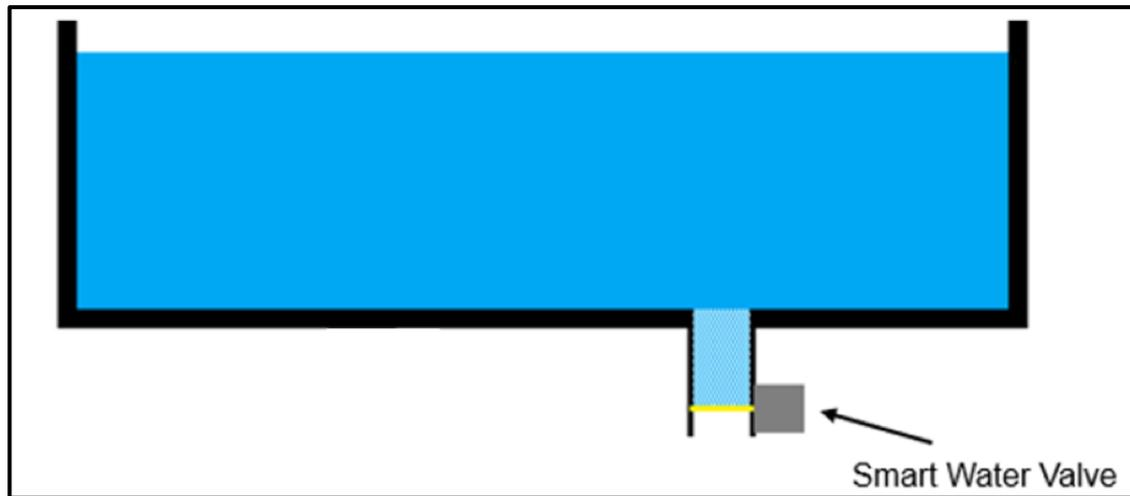
*Figure 3.1: The theorised prototype to design, suspended in air. A smart water valve is also included for a constant water release system.*
