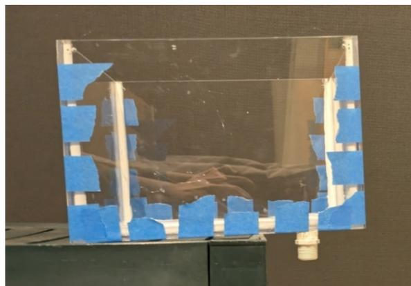
*Figure 5.15: The tank with all sides taped together left overnight for the acrylic sheets and valve adaptor to bond.*
