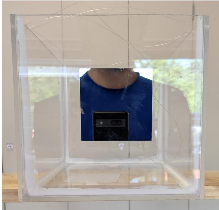
*Figure 5.16: The mirror panel applied to the side of the tank for aid in measurement purposes.*
