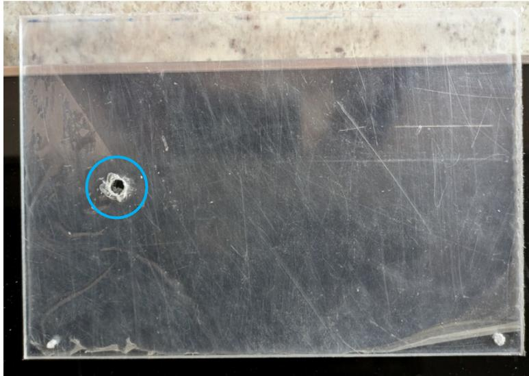
*Figure 5.14: An acrylic panel exhibiting one larger hole (circled in blue) that will be used to fit the valve adaptor.*
