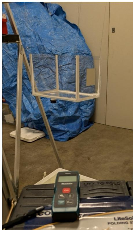
*Figure 5.19: The experimental set up of the laser measurer mounted upon a ladder pointed towards the mirror panel on the leaky tank.*
