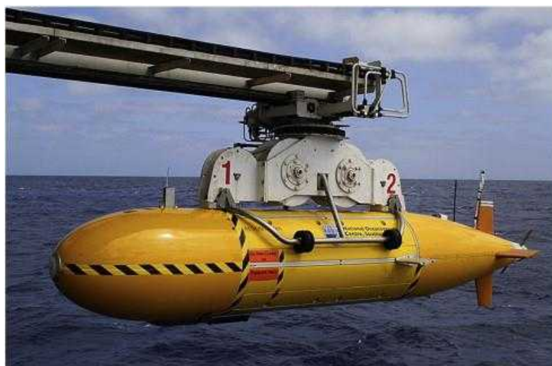
Figure 2: The UK Natural Environment Council (NERC) Autosub6000 AUV [6].
