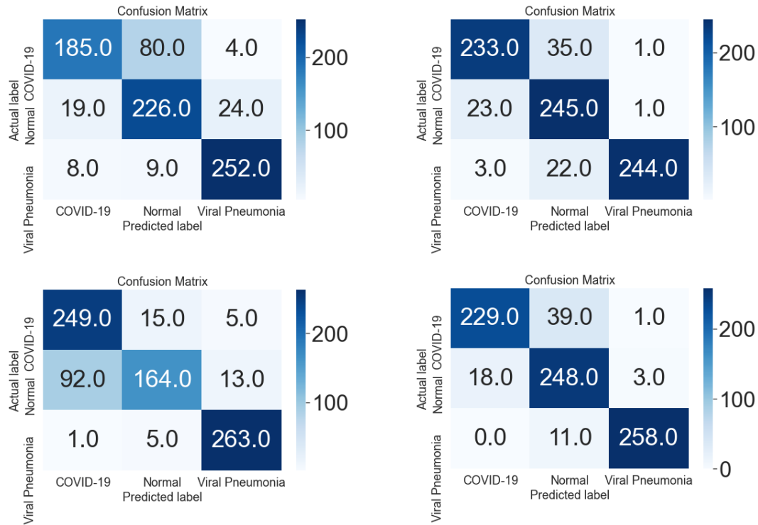
Figure 5 Confusion matrices for custom CNN (top left), VGG-16 (top right), Inception-V3 (bottom left) and DenseNet-121 (bottom right) for dataset B
